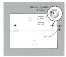
which are then etched onto the panel. These targets are located along the long axis of the panel, equidistant from the centerline. (See diagram) If targets cannot be computer generated then other methods of target placement can be custom tailored to your production needs.
